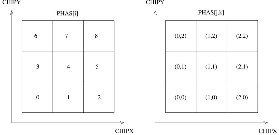
Figure 1: The relative CHIPX and CHIPY coordinates of the nine elements of a 3 pixel by 3 pixel ACIS event island (i.e. the nine elements of PHAS or PHAS\_ADJ for TIMED FAINT and CONTINUOUS CC33\_FAINT mode data). The figure on the left-hand (right-hand) side is appropriate if one (two) index is used.
