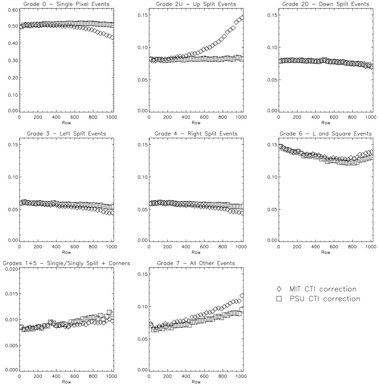
Figure 6: Ratio of events in various grades to total telemetered events as a function of row. Note that the y-axis range is different for the G0 and G1+G5 events. The MIT corrector does not change the observed event grade.
