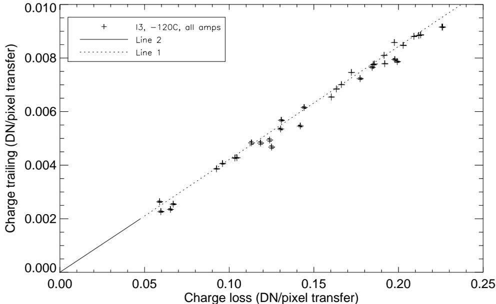
Figure 2: The piecewise-linear model of parallel charge trailing per pixel transfer for I3 (all nodes) at -120C. The Au-L line produced unreliable results and is not included.
