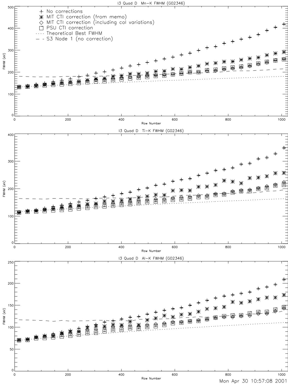
Figure 3: FWHM versus row at 5.9, 4.5 and 1.5 keV. Data corrected using the current MIT (diamonds) and PSU (squares) CTI correctors perform very similarly. Also shown are uncorrected data (+), the MIT CTI correction reported earlier (\*), the theoretical limits on I3 performance and the current performance of S3 (without CTI correction). The error bars shown are from counting statistics and are therefore very small.
