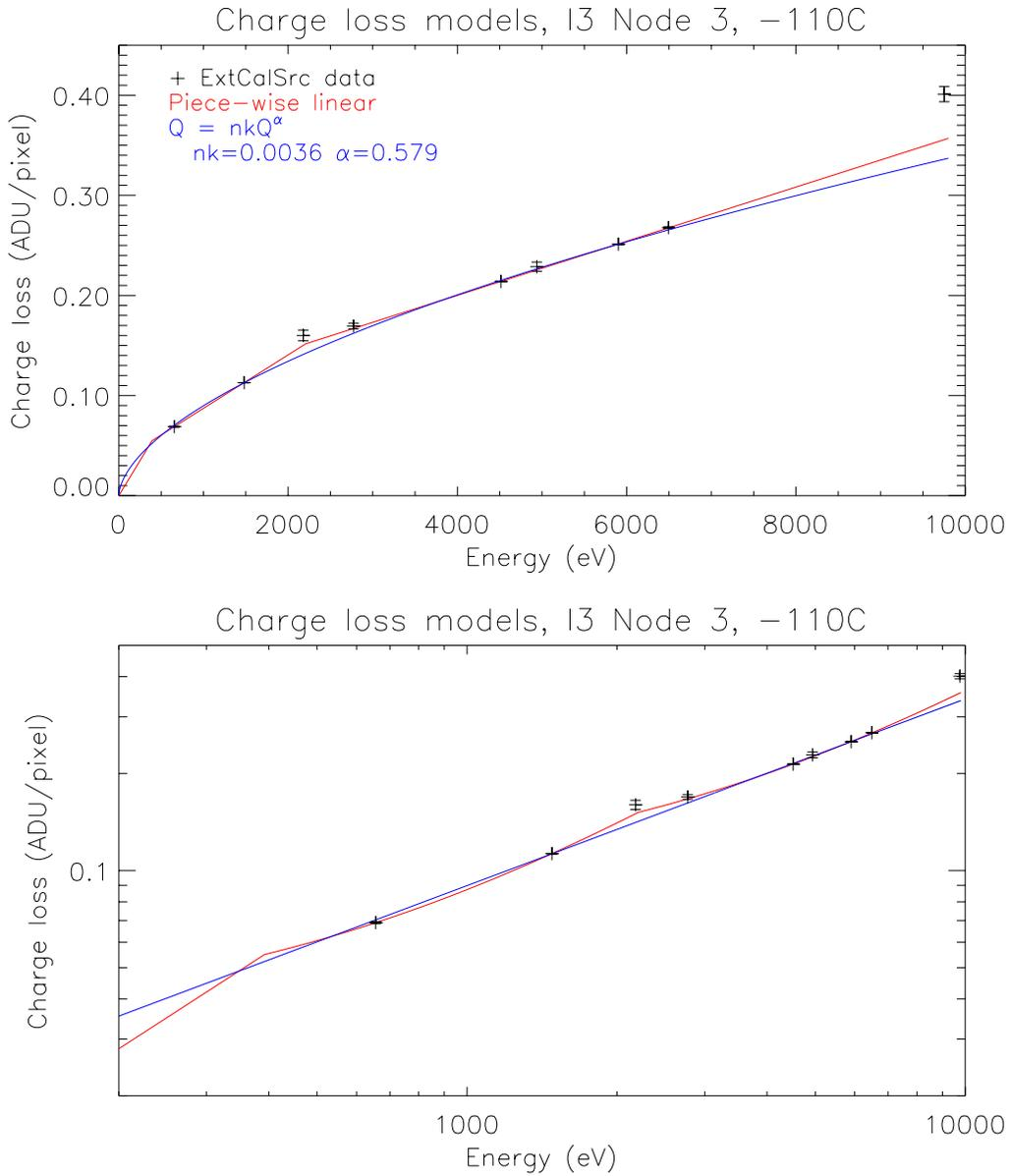
Figure 7: Comparison of the piece-wise linear (red) and power law (blue) charge loss models used by the Penn State and MIT CTI correctors in linear (top) and logarithmic (bottom) plots for a focal plane temperature of -110C. This is an example fit; other nodes and devices can be better or worse fit at high energies. Data used to calibrate this relationship are also shown (courtesy of the PSU CTI corrector group).
