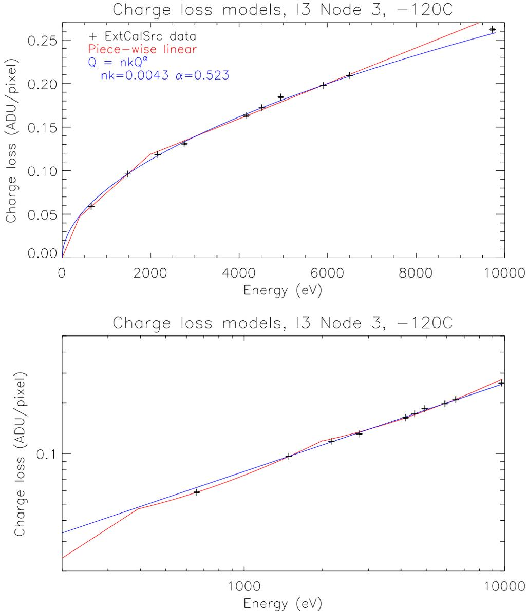
Figure 1: Comparison of the piece-wise linear (red) and power law (blue) charge loss models used by the Penn State and MIT CTI correctors in linear (top) and logarithmic (bottom) plots for a focal plane temperature of -120C. This is an example fit; other nodes and devices can be better or worse fit by either model. Data used to calibrate this relationship are also shown (courtesy of the PSU CTI corrector group).
