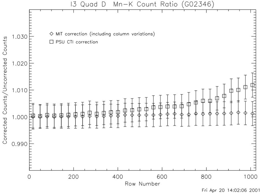
Figure 5: Ratio of corrected to uncorrected counts at 5.9 keV (G02346 events).
