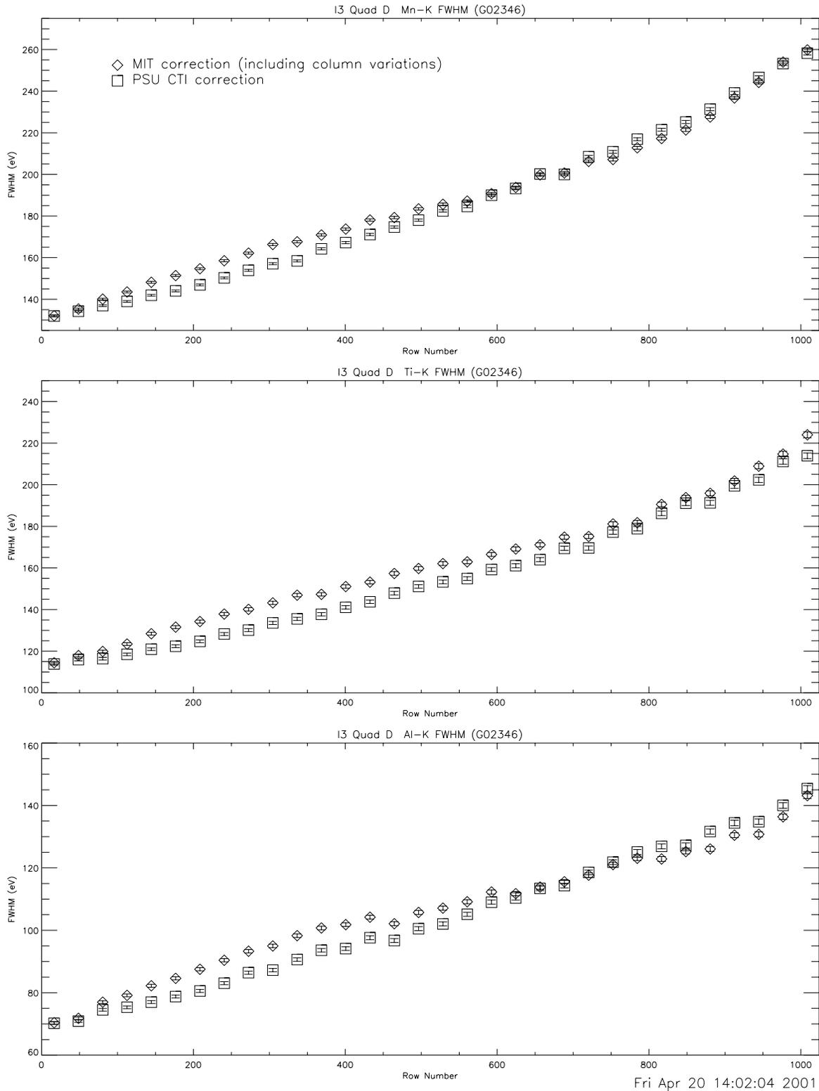
Figure 4: FWHM versus row at 5.9, 4.5 and 1.5 keV. This is the same data as Figure 3 with the y-axis range decreased to emphasize the differences in the MIT and PSU CTI corrector performance. The error bars shown are from counting statistics and are therefore very small.
