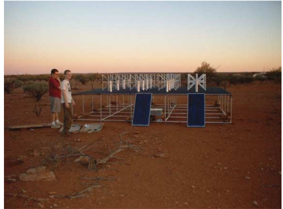
Fig. 4. This photograph shows an MWA prototype antenna being tested on site in Mileura. The antenna consists of 16 crossed dipoles, and the signals from the dipoles are combined at each antenna by a switchable analog delay line. The resulting beam is 15\text{--}45^\circ across, and can be steered by digitally switching the delay lines. Five hundred of these 16 dipole antennas will be placed in a 1.5 km array for the low frequency band of the final MWA observatory.
