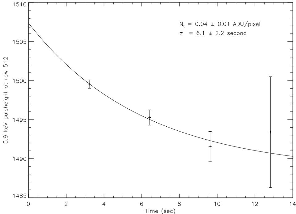
Figure 1: Fitted Gaussian peak of center pixel pulseheights at row 512 versus time between precursor and event. Data has been CTI corrected.
