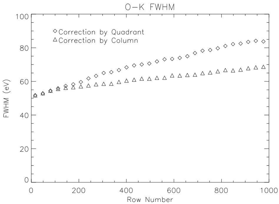
Figure 4: FWHM (eV) of the O-K line versus row number using a pulseheight correction calibrated for the entire quadrant and a pulseheight correction calibrated for each individual column.
