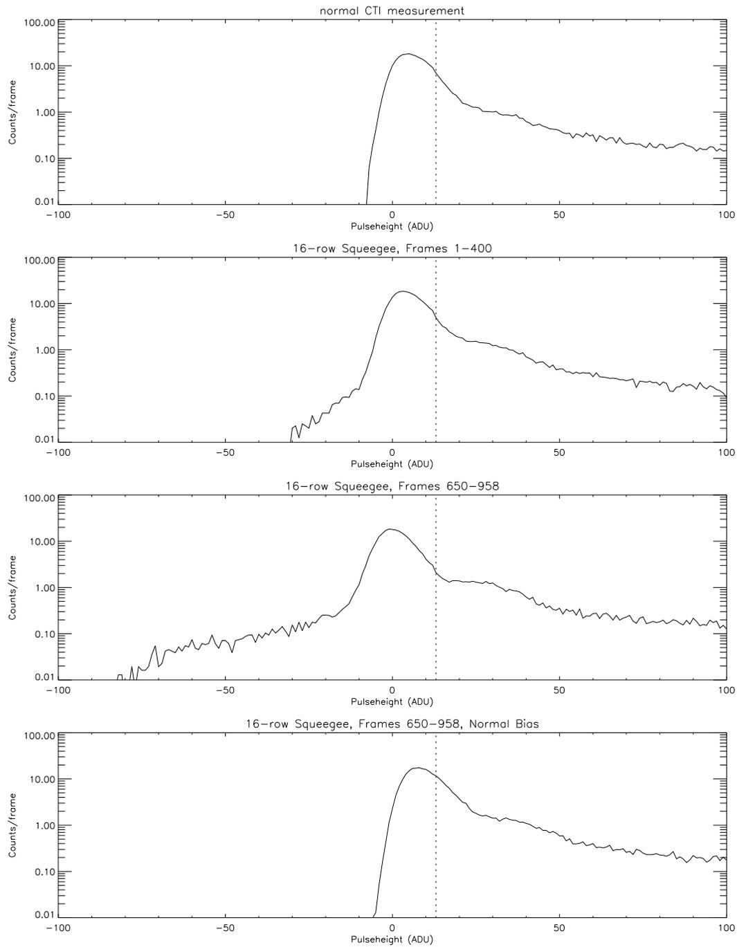
Figure 4: The distribution of pulseheights in the top pixel of each event island. From the top to the bottom, a normal CTI measurement, exposures 2-400 of the 16-row squeegee test, exposures 650-958 of the 16-row squeegee test, and exposures 650-958 of the 16-row squeegee test using the bias frame from the normal CTI measurement.
