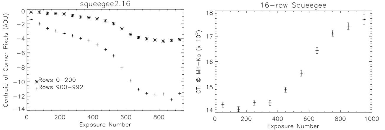
Figure 3: The change in corner pixel values during the squeegee tests is much larger at the top of the CCD (near the squeegee) than at the bottom of the CCD (near the framestore). (Left) The bottom 200 rows show less bias decay than the top 92 rows. (Right) This differential charge decay increases the measured CTI
