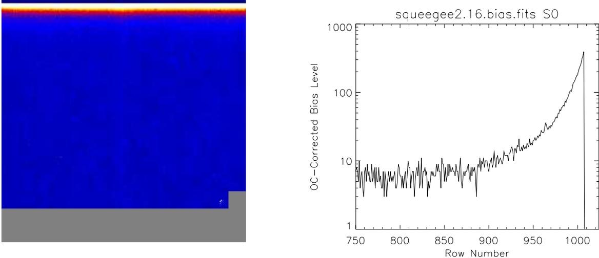
Figure 1: Characteristics of the squeegee mode bias frame. (Left) Image of overclock-corrected bias frame from 16-row squeegee mode test. (Right) The overclock-corrected bias level along column 400, a representative column, showing the squeegee spillover.
