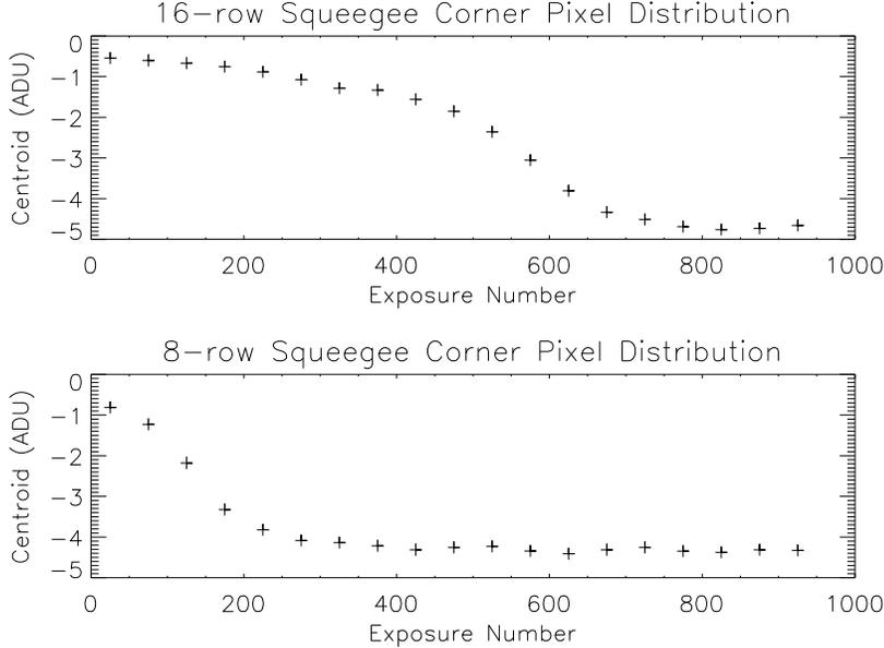
Figure 2: Time-dependence of the centroid of the corner pixel distribution for both the 16-row and 8-row squeegee tests. The negative values for the centroids indicates that the original bias frame has a higher bias level than the exposures and that this excess charge is slowly decaying away.
