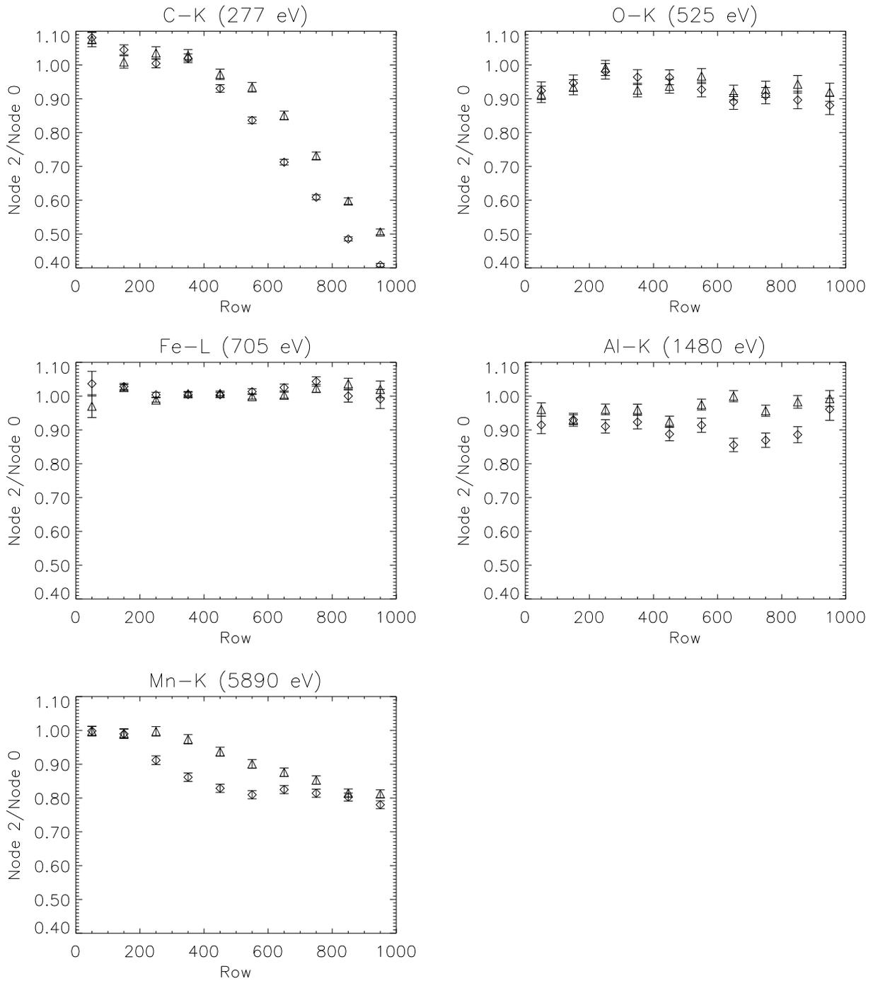
Figure 2: Relative QE as a function of row for each spectral line at -110 C ( $\diamond$ ) and -120 C ( $\triangle$ ).
