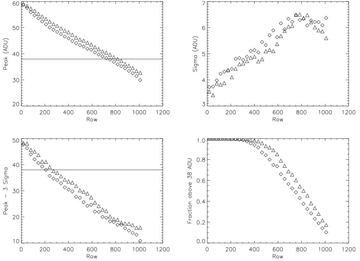
Figure 3: Results of Gaussian fits to the C-K line (277 eV) in the damaged portion of the CCD at -110 C ( $\diamond$ ) and -120 C ( $\triangle$ ). See the text for explanation. The horizontal line indicates the flight instrument event threshold of 38 ADU.
