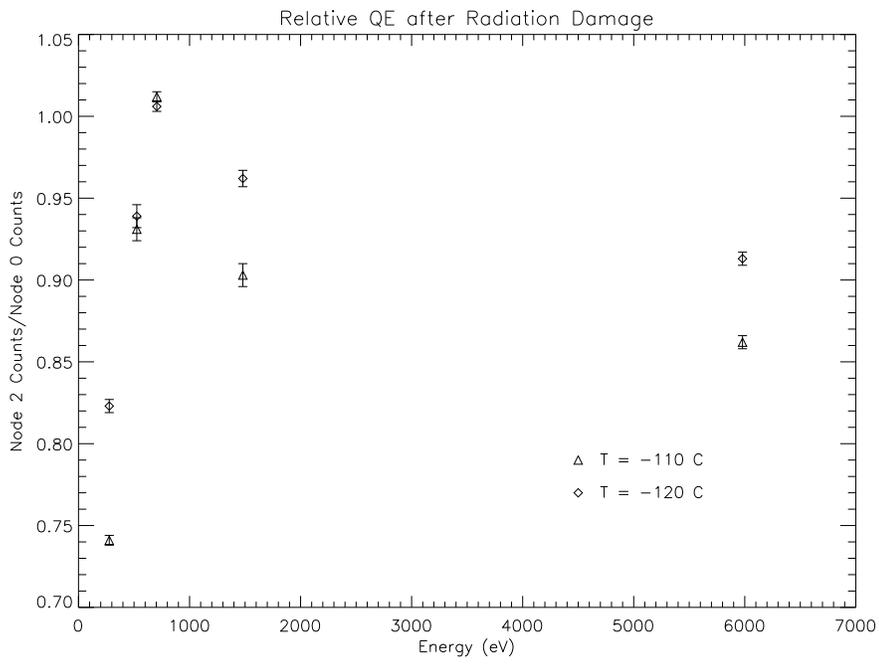
Figure 1: The relative QE of the radiation damaged node to the undamaged node at a temperature of -110 and -120 C.
