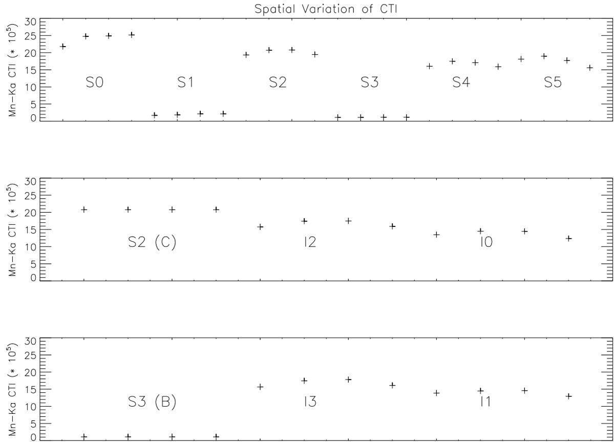
Figure 1: CTI variability for three cuts through the ACIS focal plane. The position coordinate is not a real distance measurement. The 'humped' structure seen for all the FI CCDs is not a result of non-uniformity in detector damage.
