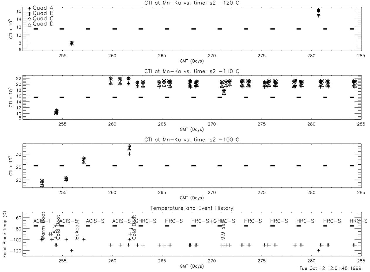
Figure 1: CTI measurements at the Mn-K $\alpha$  (5.9 keV) line at temperatures of -120, -110 and -100 C. The bottom panel represents a history of events and temperature changes. The solid horizontal lines represent when Chandra was passing through the Earth's radiation belts, a possible location of damaging particles.
